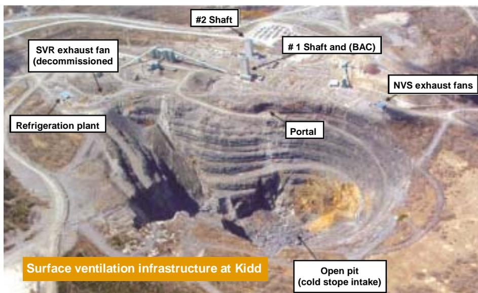
air with the previously-cooled rubble, cools the air being delivered to the underground workings. Airflow through the cold stope is collected in a raise and delivered to the 2,800 level, where the flow is controlled through two 54 in 250 HP axial fans. These fans, in turn, deliver the cooled air to the top of #3 Shaft (internal hoisting shaft) on the 4,700 level for distribution in #3 Mine and, in particular, Phase I.
