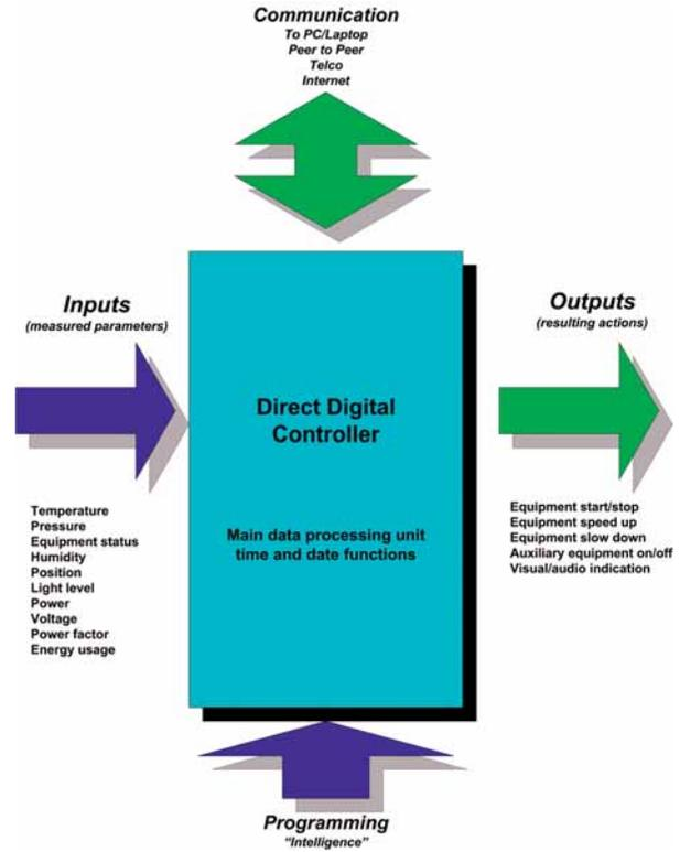
Figure 3: Direct digital controller
